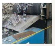
The 360° magnet system retains extracted iron, discharging it behind the centre line of the pulley, whilst the clean product follows its natural trajectory. All units are available with either ferrite or rare earth magnet
